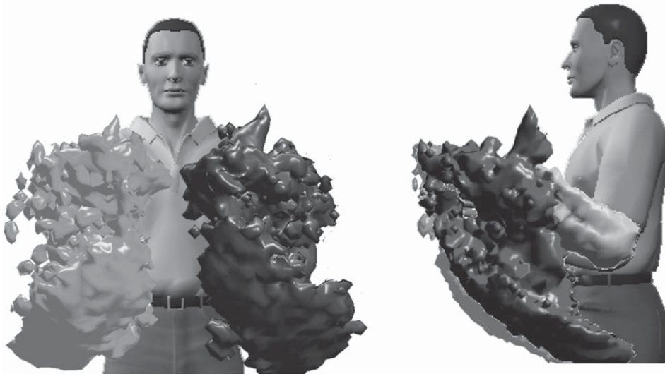
Fig. 2. 3-D probabilistic clouds of hand and elbow positions in healthy adults. Front (left) and side views (right) show the outer boundaries of regions that represent 90% of all locations visited by a typical subject's wrists and elbows. Courtesy of Daniel Wolpert, modified from Howard et al. (2016).
